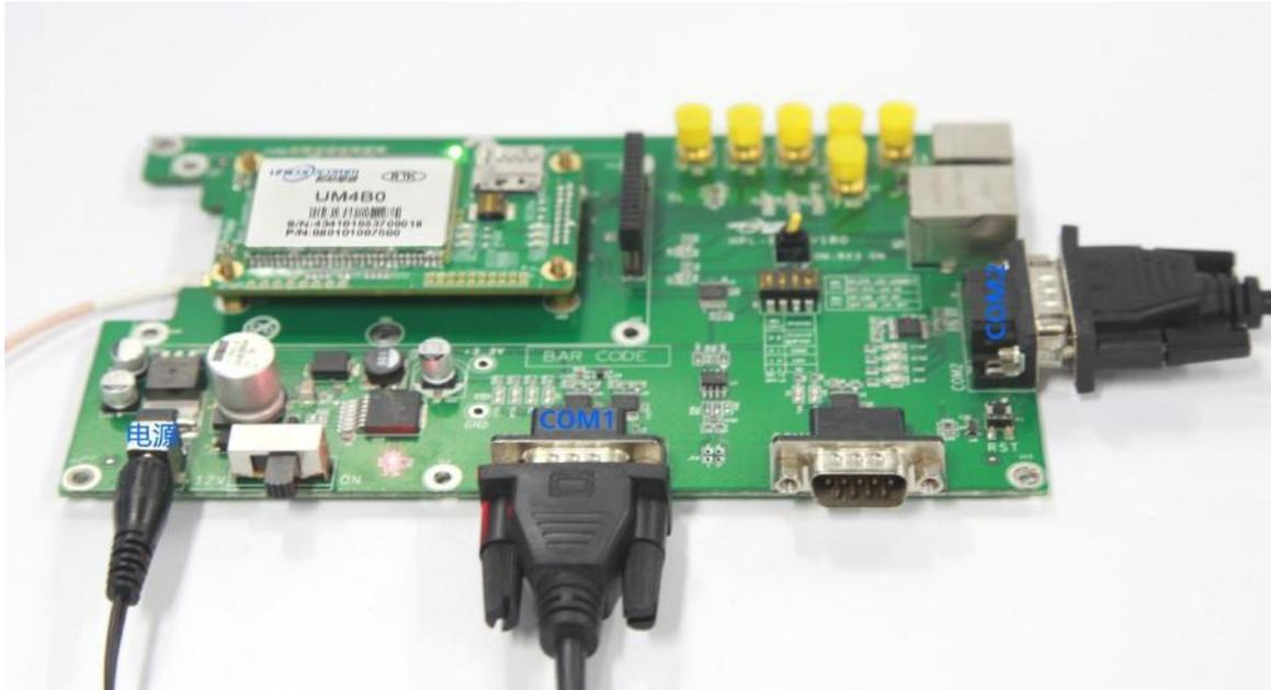
Figure 4-3 Connect the Serial Port
