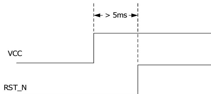
Figure 3-4 UM482 RST\_N Timing Sequence
