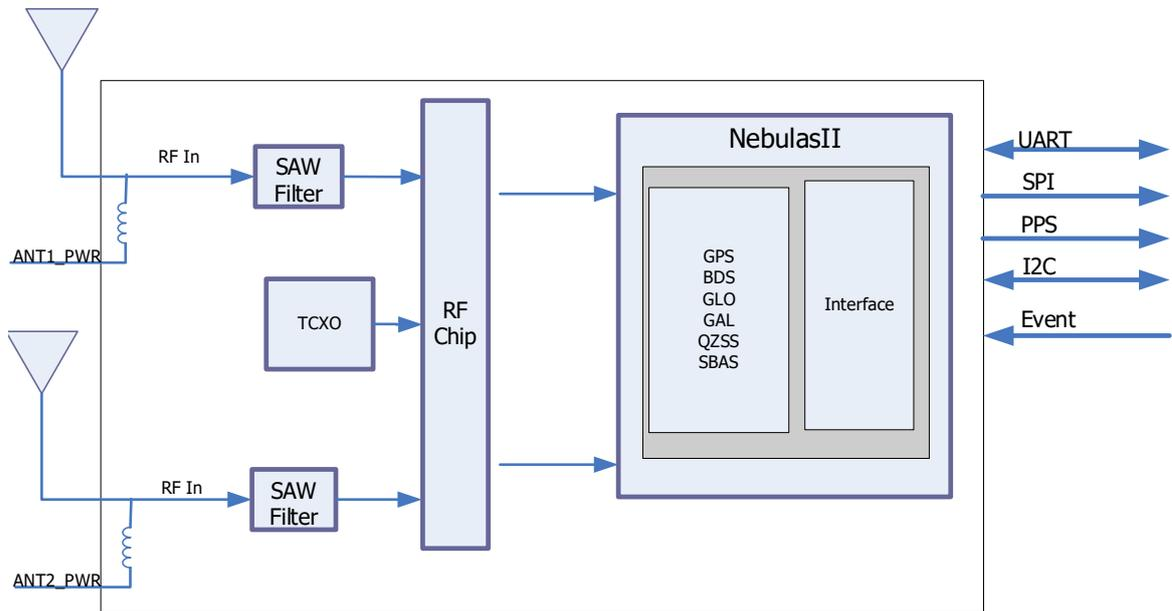
Figure 1-2 Block Diagram
