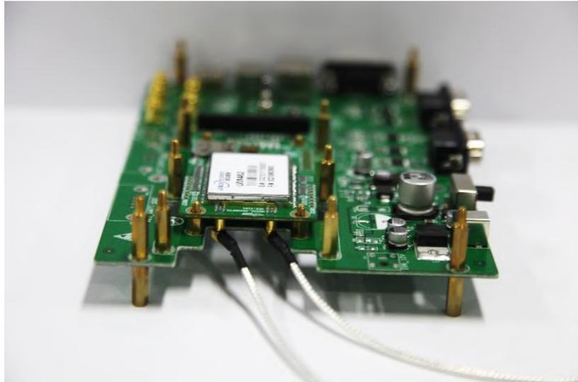
**Figure 4-3 Connect the Antenna**
