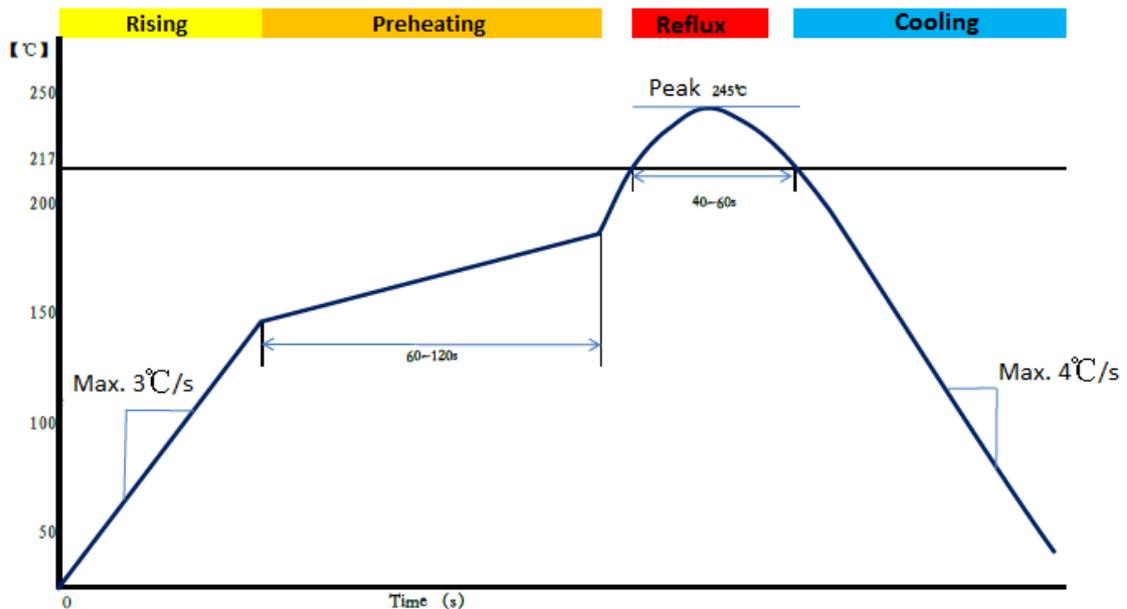
Figure 8- 1 Soldering Temperature
