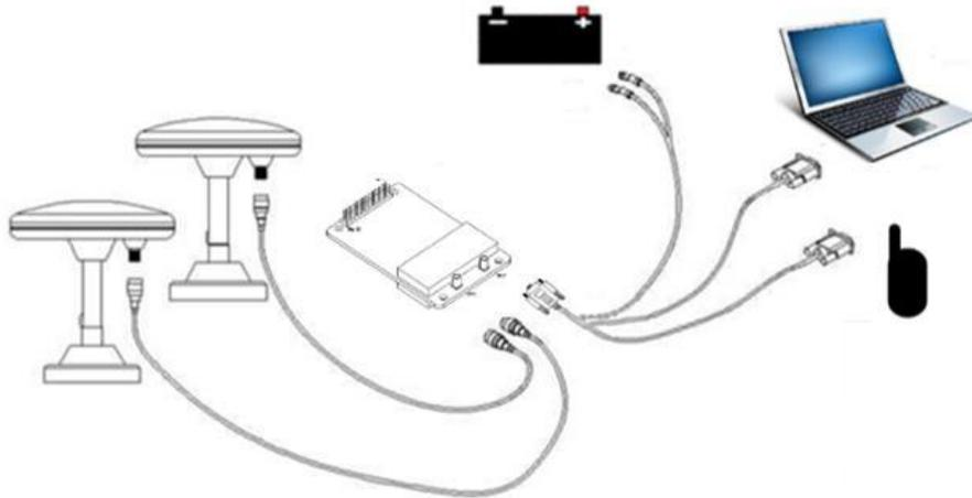
**Figure 4-1 Typical Installation of UM482**
