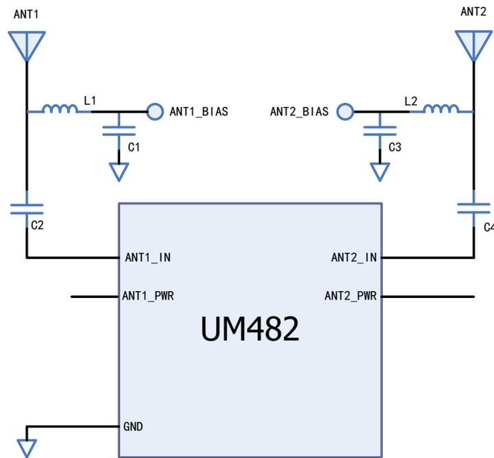
Figure 3-5 UM482 External Antenna Feed Reference Circuit
