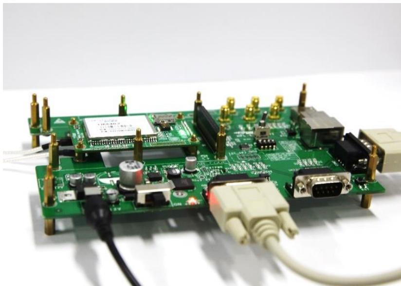
**Figure 4-4 Connect the Serial Port**
