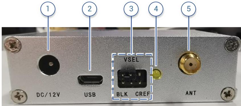
Figure 3-1 Interfaces & Indicator on UC6226NIS EVK (Front Panel)
