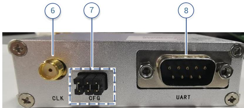
Figure 3-2 Interfaces & Indicator on UC6226NIS EVK (Rear Panel)
