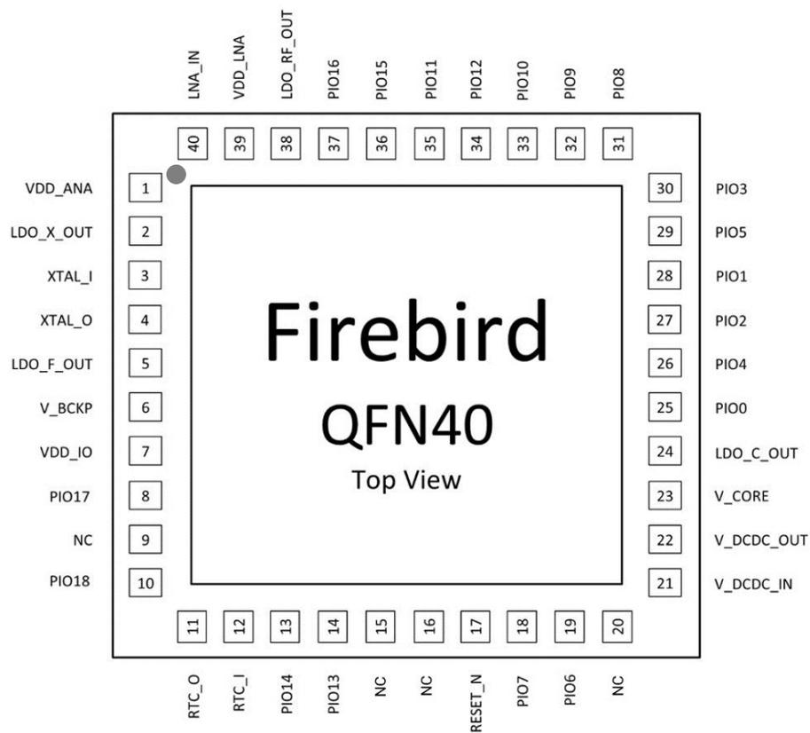
Figure 6-1 QFN40 pin diagram
