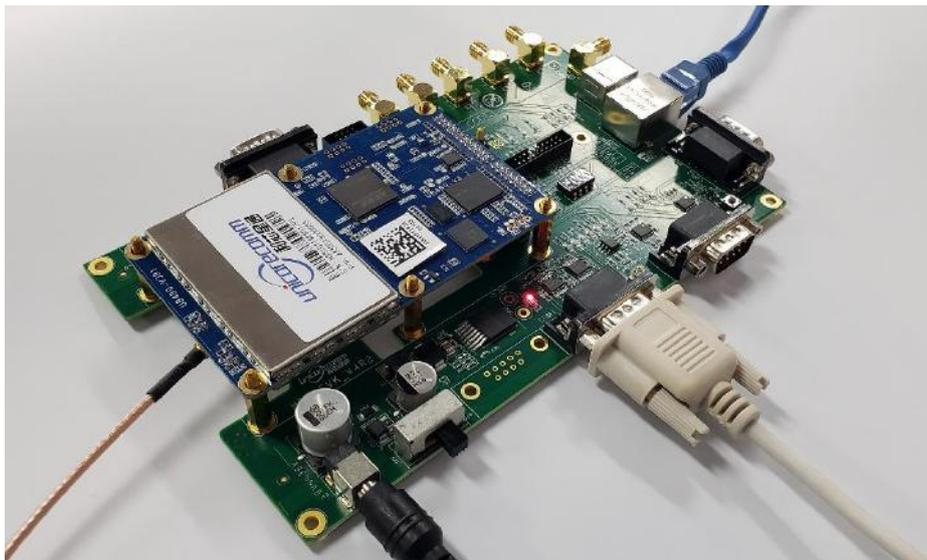
**Figure 3-5 Installation Step 3**
