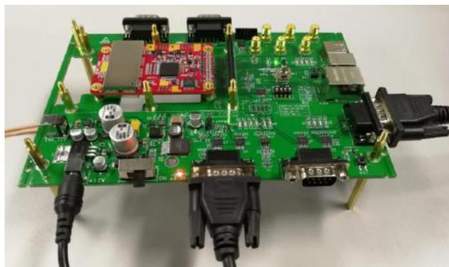
**Figure 4-3 UB482 Serial Port, Power Connection**
